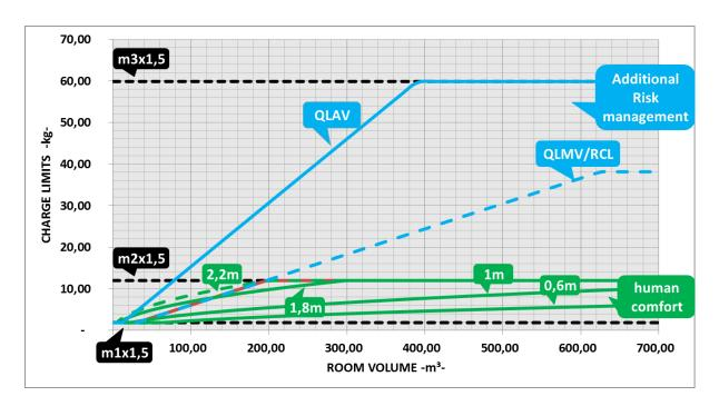
To clarify the additional measures, we can use the following diagram to explain the different types of additional measures used across the standard
